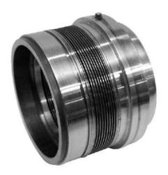
MBH Mechanical seal is hook sleeve design for handling heat transfer media & high temp hydrocarbons. The seal is self-cleaning without springs. Metal bellow seals are pressure balanced seals.
