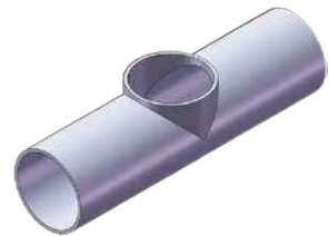
SMS 9WO Welding Cross Without Straight-End
